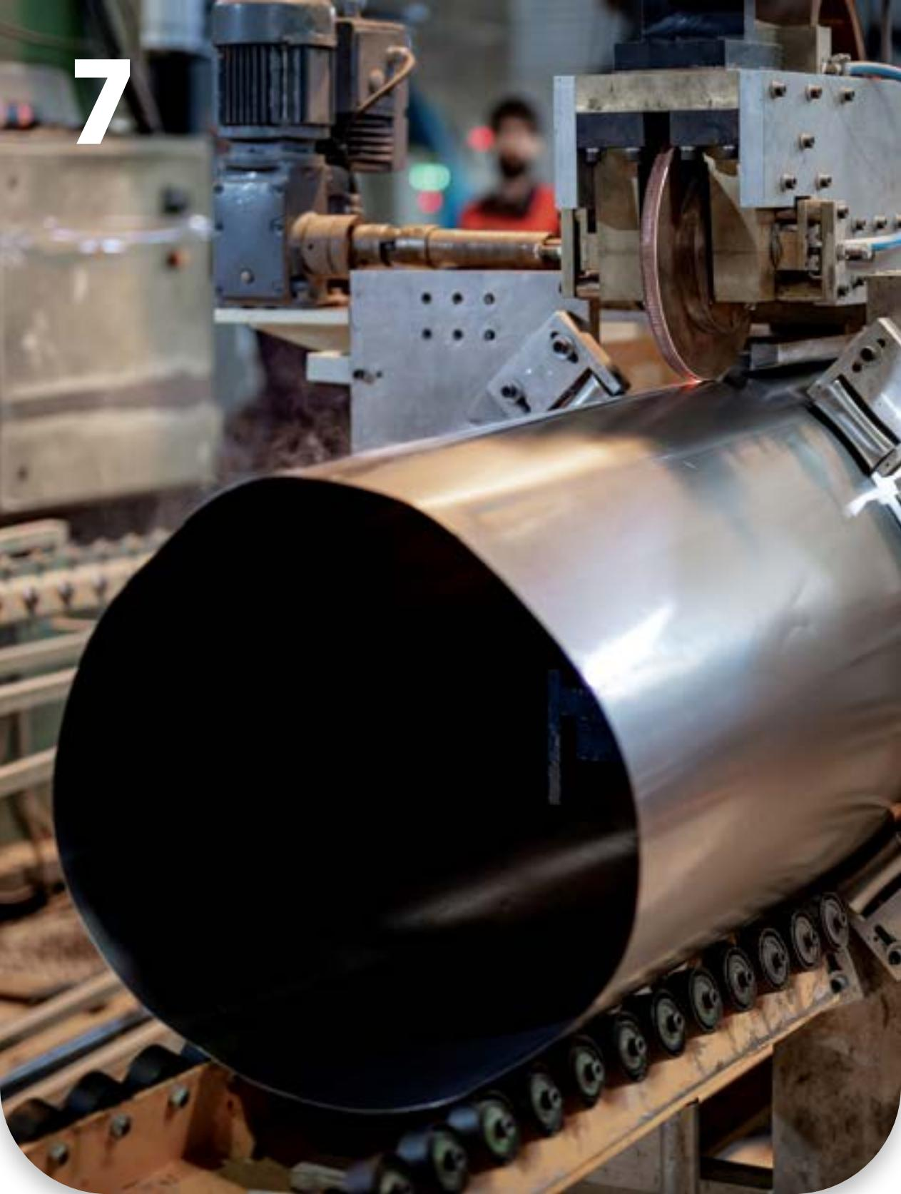
The technology and design of the companies machinery have resulted in a particular system synergy, leading to a more than 85% of the entire production line being automated, and the related outcome has resulted in improving the quality of drums in shaping a high-quality product for export.
