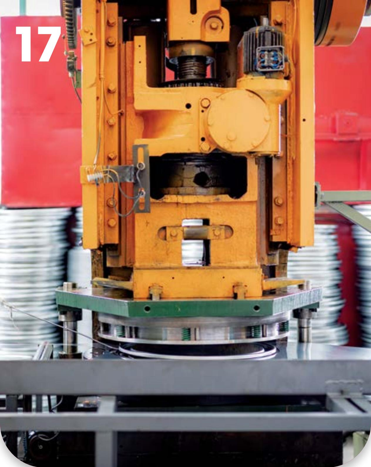
To produce drum doors, a desired molding has been developed, which is produced on a daily basis with a high production volume using the stamping mechanism and a matrix. Upon the request of the customers and intending to improve the quality, it is possible to use special insulation tapes inside the drums to ensure a better seal for certain products requiring certain levels of humidity.
